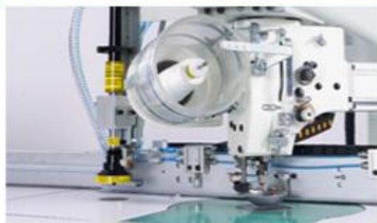
Laser function, can be used to open high-end down jacket zipper pockets welting, suit pocket welting, etc.
